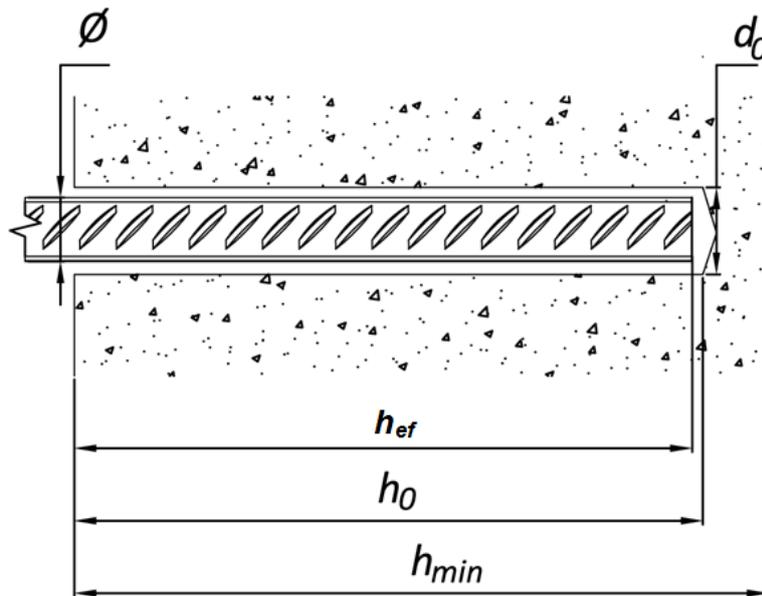
**Table B3: Installation parameters – rebar**
