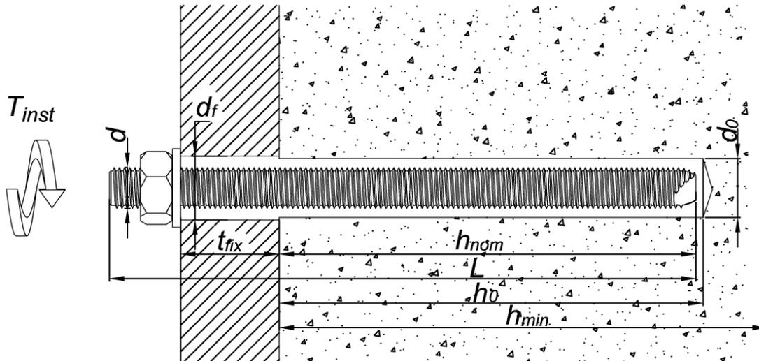
**Table B1: Installation parameters – threaded anchor rod**
