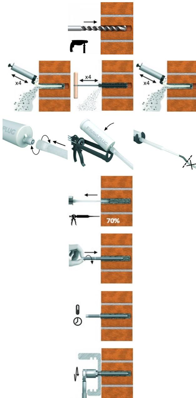
1. Drill the hole to the required diameter and depth (hammer drilling for solid masonry and rotary drilling for AAC).
