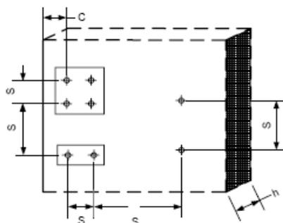
**Table C11: Brick No. 1, 2 and 3 - edge distance and spacing for tension load**
