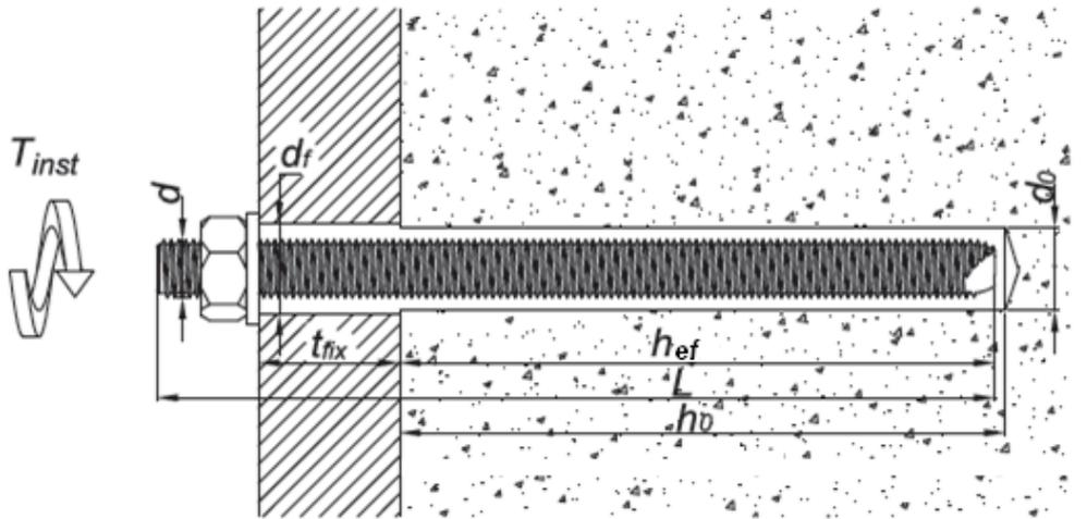
**Figure A2: Anchor rod with perforated sleeve – installation in perforated masonry**
