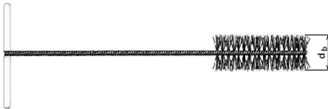
**Brush diameter for solid masonry**
