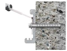
5. Place the dispensing nozzle in the opening of the sealing ring. Fill the annular gap with resin.
