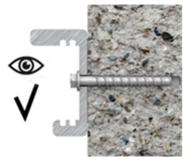
4. Finish screwing when the screw head is in full contact with the fastened element/substrate. The screw head must not be damaged.
