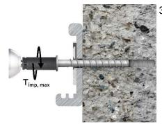
3. Place the sealing ring on the fixture. Screw the concrete screw into the hole using an impact wrench and an appropriate impact socket. Tighten until the element is pressed to the surface. Installation using any impact wrench with a tangential impact.
