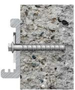
Finish screwing in when the screw head and the ring are in contact with the fastened element/substrate. The screw head must not be damaged.
