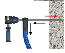
2. Clean the hole (blow dust at least 4 times with the hand pump). When using a dust-free drill bit (1b), it is not necessary to clean the hole.
