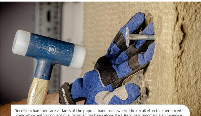
Recoilless hammers are variants of the popular hand tools where the recoil effect, experienced while hitting with a conventional hammer, has been eliminated. Recoilless hammers also minimise the straining of arm joints and muscles, which makes them far superior in terms of handling comfort and safety, while they prove particularly useful when performing jobs that require
