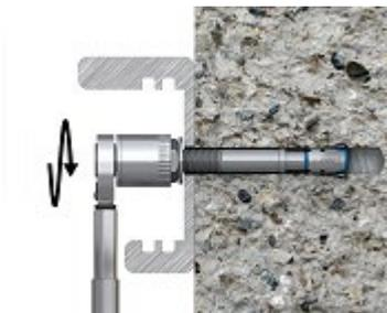
Tighten to the recommended torque
